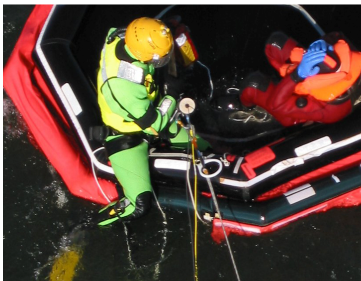
The GLR1000 is connected to the raft and the guideline run through the GLR1000. No entangling in the life raft.
